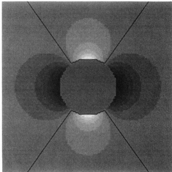
FIG. 1. Relative changes (coded in half-tone steps) of the specific volume  $\delta v(\mathbf{r})/v_0$  in a system consisting of a spherical grain in an isotropic embedding matrix subject to a uniaxial strain. The cut is taken through the center of the sphere along the plane  $z=0$  containing the strain axis.
