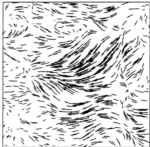
FIG. 4. The displacement  $\Delta \mathbf{U}(\mathbf{r}) = \mathbf{U}(\mathbf{r}) - \mathbf{U}_0(\mathbf{r})$  associated with the elastically deformed cluster shown in Fig. 3. Length and direction of the arrows refer to the absolute value and the direction of  $\Delta \mathbf{U}(\mathbf{r})$ , respectively.
