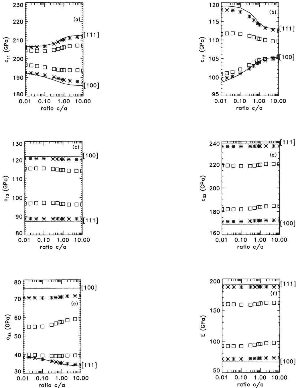
FIG. 10.  $c/a$  dependence of the elastic moduli as in Fig. 8 for fiber textures exhibiting a finite spread around the ideal orientation [100] and [111]. The latter refer to the solid curves. Results marked by asterisks and squares relate to the smaller and larger spreads, respectively.
