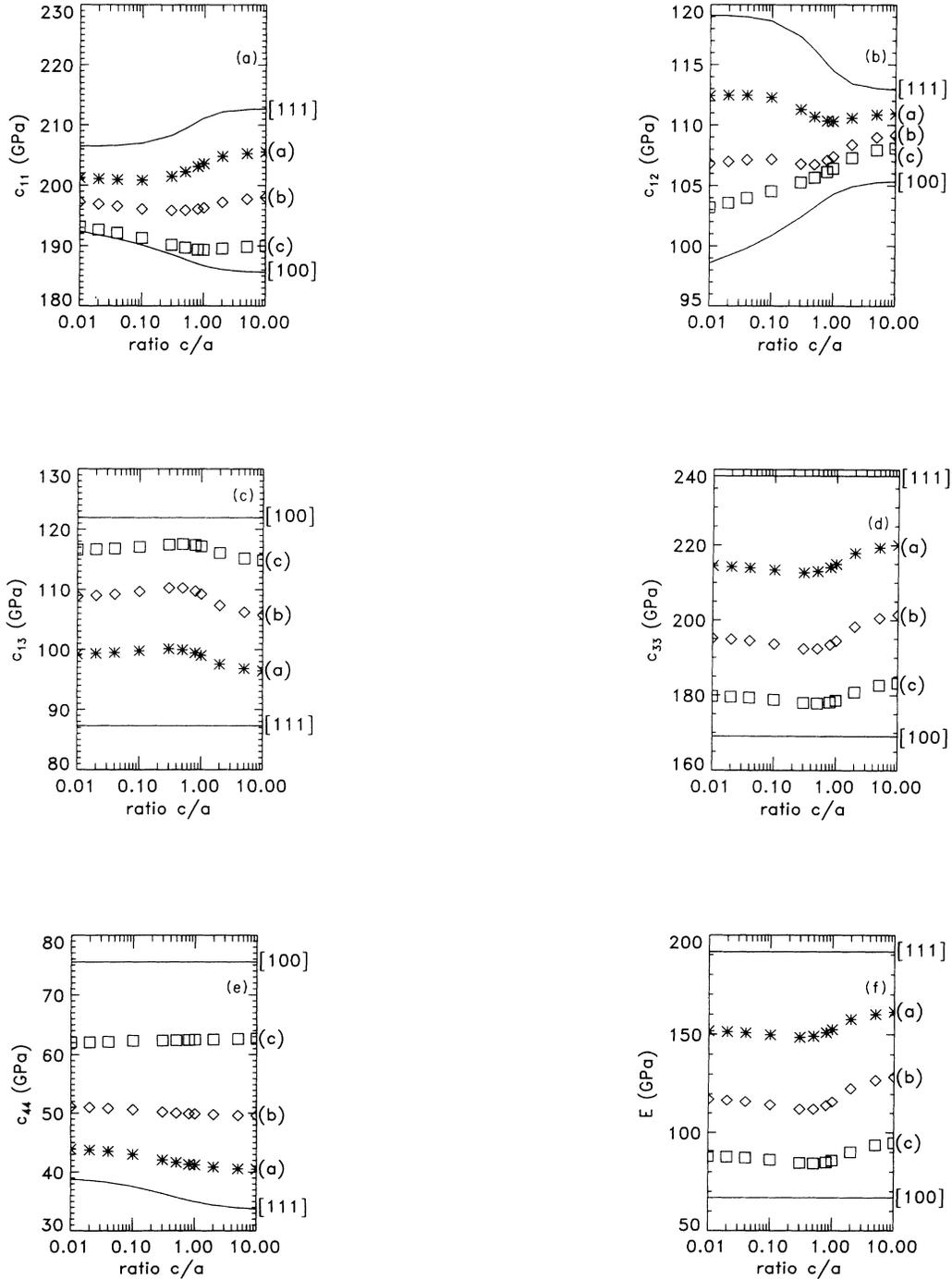
FIG. 9.  $c/a$  dependence of the elastic moduli as in Fig. 8 for a composite fiber texture of copper metal. The assumed percentages of the orientations are indicated as a parameter: (a) 23,2% [100]/76,8% [111]; (b) 45,6% [100]/ 54,4% [111]; (c) 68,8% [100]/31,2% [111]. The upper and lower solid curves refer to the pertinent ideal orientation.
